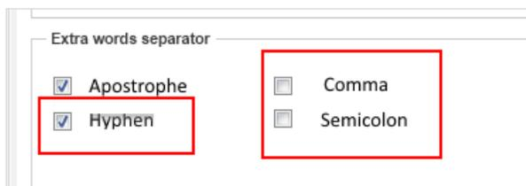
If Hyphen, **Comma** or Semicolon is enabled as an extra words separator on the TM, the enabled character is managed as a word separator. Words separated by the character without space are counted as several words.
